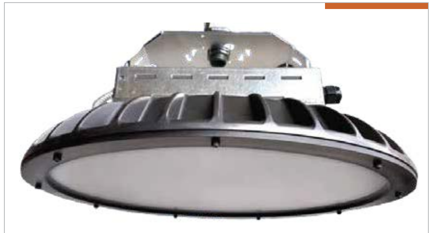
The housing of SLP Lighting's CircLED™ high bay fixture acts as a heat sink and is injection molded with Makrolon® TC8030 polycarbonate.
